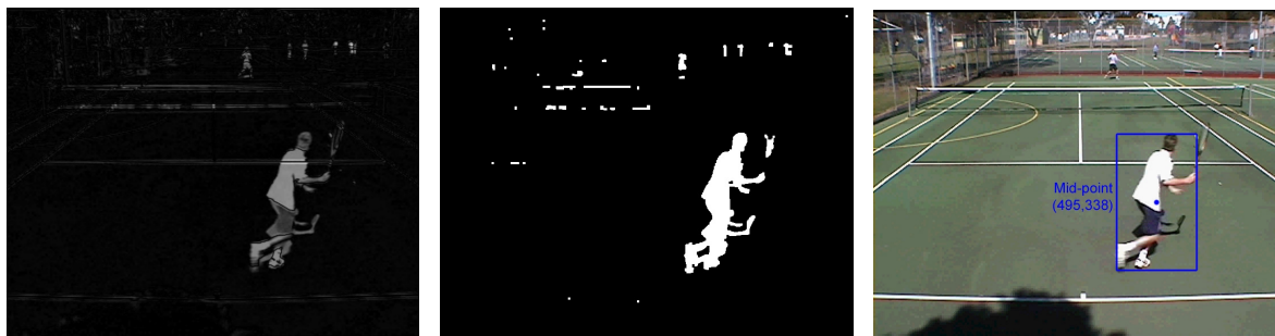
Figure 1: From left to right; the difference image produced from the pixel-by-pixel difference of a frame with the background reference frame. The difference image after thresholding and morphological filtering. The original frame with the player's position confirmed by identifying the bounding box of the blob that represents the variation in the difference image due to the player.
