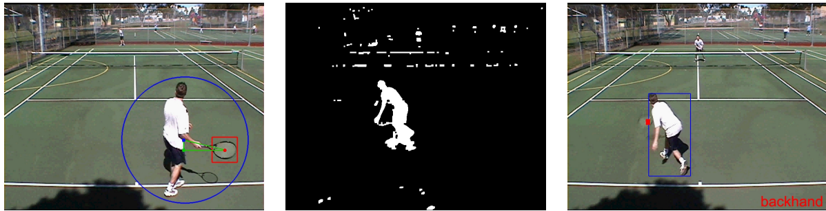
Figure 2: Left: The maximum possible racquet head size just fits into the square bounding box in red. A maximum allowable radius from the mid-point of the player is illustrated in blue. The green right-angled triangle formed from the mid-points of the player and the racquet is used to calculate the distance of the racquet from the player. Middle and right: A blob representing the racquet is found on the left of the player, thus the stroke is recognised as a backhand ground stroke.
