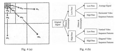
**Fig. 4.** (a) Three Levels Wavelet Decomposition of the Video Sequence (b) Wavelet Decomposition of the 2-D Wavelet Packet Transform for the Video Sequence
