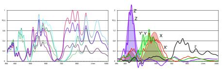
Figure 6 6-channel triple diode color sens∎r: measured spectral response and corrected functions with CIE XYZ for comparison
