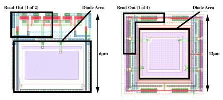
Figure 10 a) Dual Junction Photo Diode and b) Triple/Quad Junction Photo Diode; layout sample with circuitry for read-out
