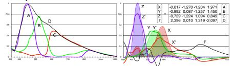
Figure 4 4-channel color sensor: measured spectral response & corrected functions
