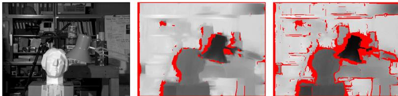
**Fig. 1.** Occlusion detection and object separation. One image of the stereo pair (left), disparity map with occlusions marked red (middle), and disparity map with occlusions and object separation marked red (right).
