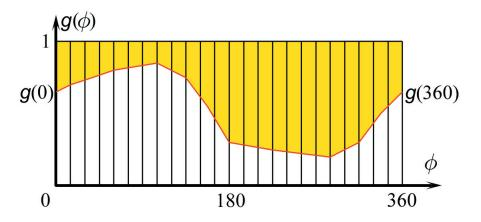
**Fig. 4.** A look-up table. The curve line from g(0) to g(360) is the value of function  $g(\phi)$ , and the area above the line is the valid area. Note that g(0) = g(360).
