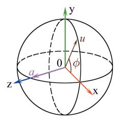
Fig. 2. Arrangement of local coordinate frame and the parameterization of vector  $\boldsymbol{u}$ .
