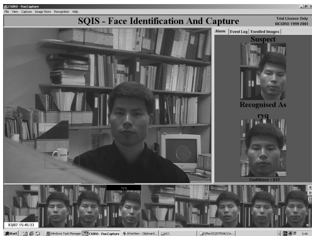
Figure 2. The SQIS TM system interface. This is the main operation screen which consists of live video, timeline showing the captured images and the enrolment/alarm screen.
