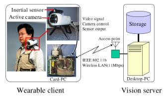
Figure 1. Prototype system for VizWear-Active.
