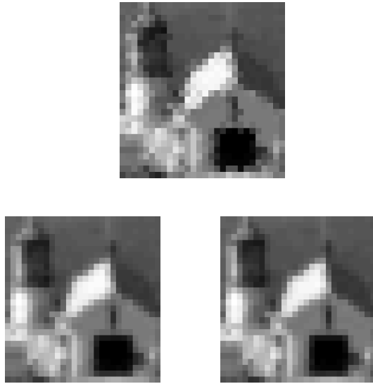
Figure 4 – Enhancement results by interpolation. From top to left and right: Nearest neighbour, Linear and Cubic
