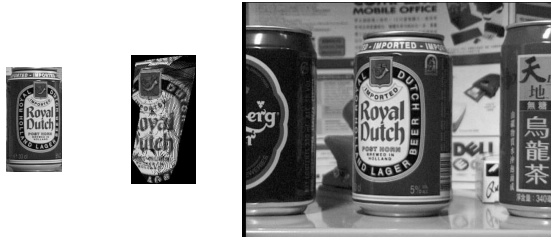
Figure 6: The warping of Template b (only the portion matched with View 2) from the viewpoint of the current view to the viewpoint of View 2. The warping is essential for cross-correlation comparison, in the same viewpoint, of the selected template (of the current view) with the candidate view (View 2 here).
