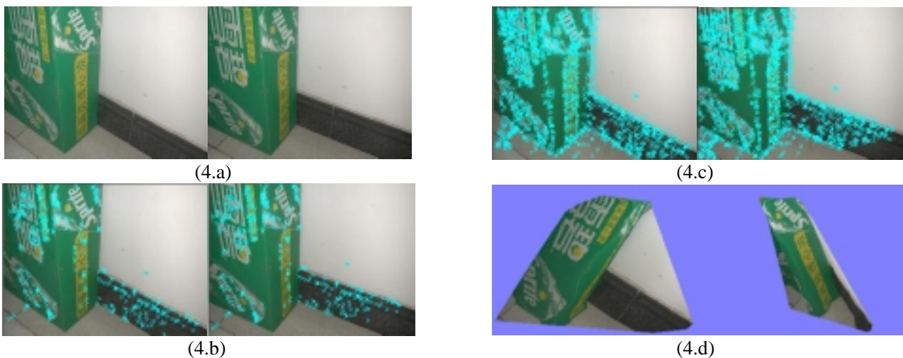
Figure 4. (a) A pair of images about a green box taken from our lab. (b) the results of sparse matching (marked by blue cross). (c) the results of semi-dense matching. (d) the results of 3D reconstruction from sparse matching(left) and semi-dense matching(right).
