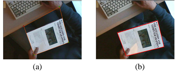
Figure 5. Comparison between (a) tracking with edges and (b) tracking with side statistics.
