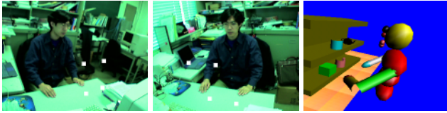
Figure 2. (left) Four landmark points of virtual objects. They are overlaid in two real images. (right) The virtual objects (cube, cup, cylinder and teapot).
