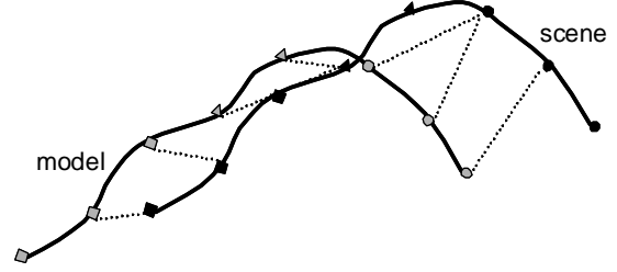
Figure 3. Point mates using point-point distance metric with reflectance strength values. Different shape marks indicate different reflectance strength values.
