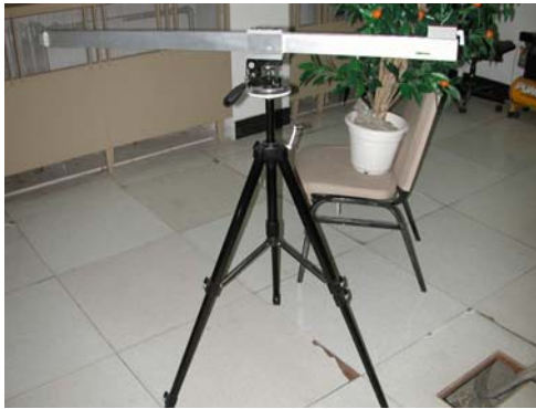
Fig 8. Our 1D camera self-calibration system: with a straight bar mounted on a tripod.
