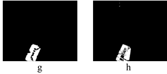
Figure 3. An example of object detection, (a) a frame in an indoor video sequence, and the lighting has changed largely, (b) the image of r_r , (c) the image of r_g , (d) the image of r_b , (e) the reference image, (f) the detection result of the first step, (g) the result after integrating connectivity constraint, (h) the detection result using conventional background subtraction
