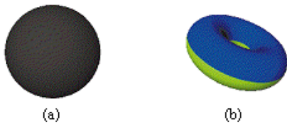
Figure 2. Mesh partitioning using watershed algorithm. (a) sphere (1 region). (b) torus (2 regions).
