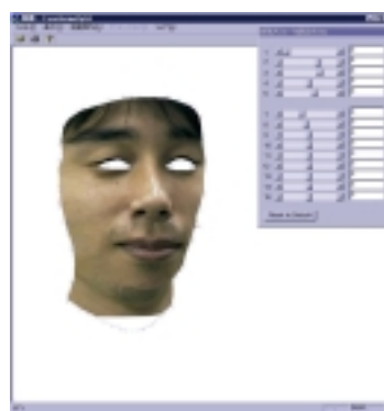
Figure 11: Changing a textured face model by changing the coefficients of the 3D eigenfaces
