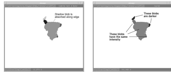
Figure 9. Absorb shadows in labelled image (a) and average luminosity of parts (b).
