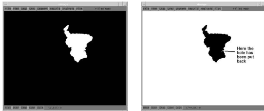
Figure 4. Background filling (a) and hole removal (b).
