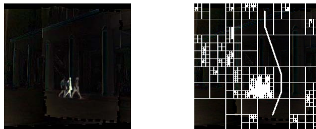
Figure 4. Best path detection in quad-tree difference image. Left image is the relative difference image of a pair of registered images, only regions of moving objects have large intensity. Right image is the result of quad-tree decomposition, white thick line segments shows the best path detected.
