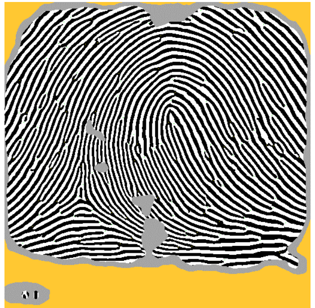
Fig. 7 - Segmented print into background (clear gray), noisy areas (dark gray), ridges (black) and valleys (white)
